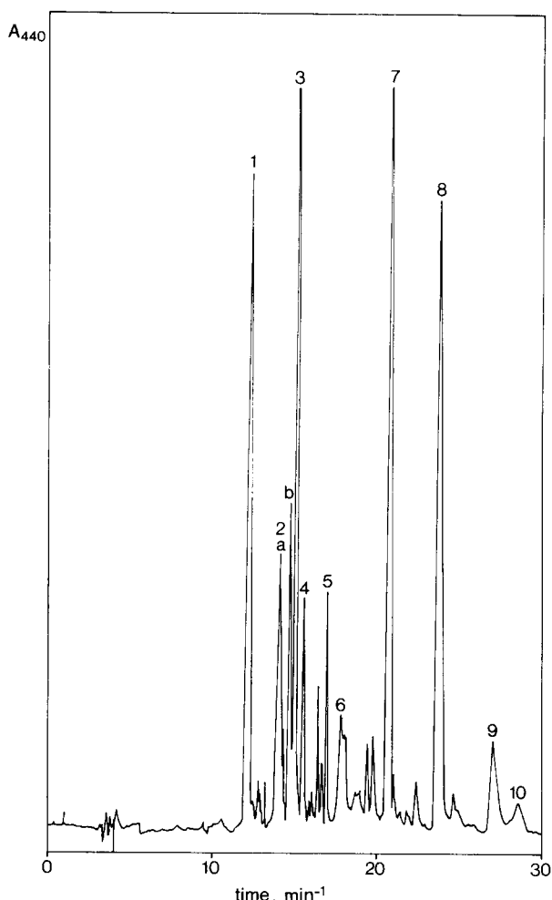
Fig. 1. HPLC-scan of the photosynthetic pigments from Mantoniella (for separation conditions, see Materials and Methods). The identification of the different fractions is as follows: 1, Chl c *; 2a, neoxanthin; 2b, violaxanthin; 3, prasinoxanthin; 4, prasinoxanthin-epoxide; 5, lateoxanthin; 6, not identified; 7, Chl b ; 8, Chl a ; 9 and 10, carotene.
