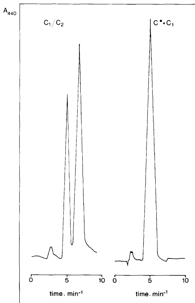
Fig. 6. HPLC scans of Chl c_1/c_2 and the cochromatography of Chl c^* and Chl c_1 in the RPX-system (see Materials and Methods).
